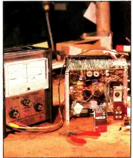
One of the first steps in determining the cause of the problem is testing transistors in-circuit.
